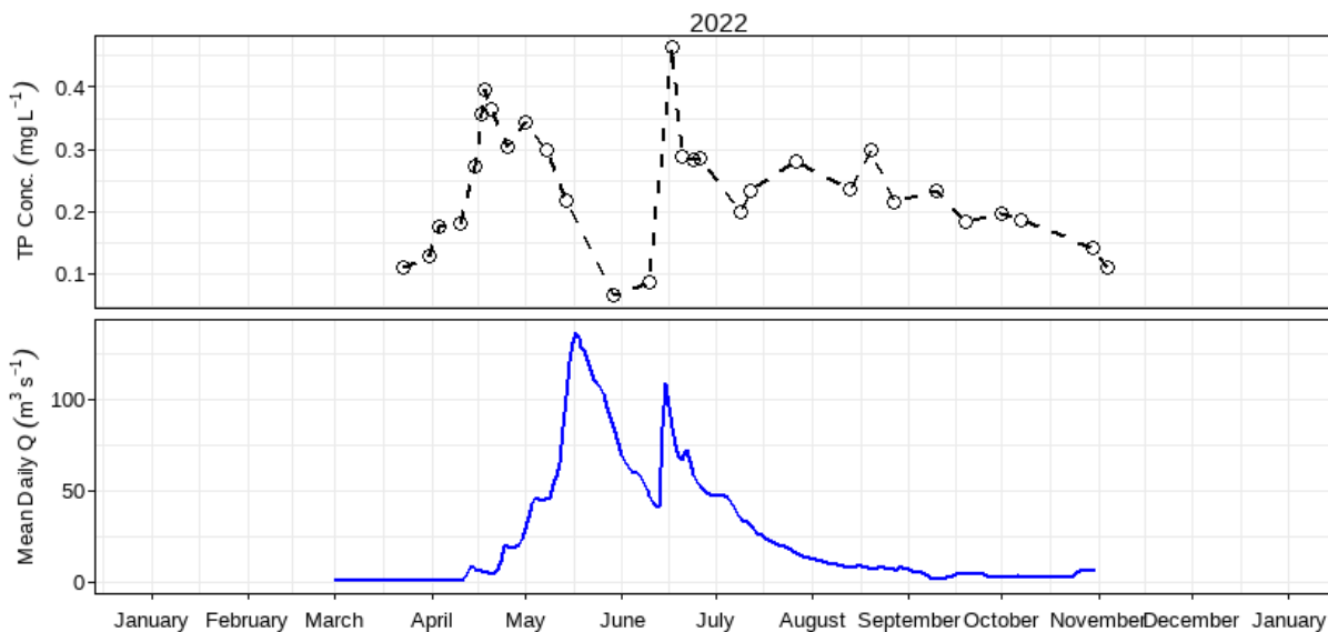
Figure 12: Mean daily discharge (m 3 s -1 ) and total phosphorus concentration (mg L -1 ) over the 2022 sampling season at Little Saskatchewan River near Rivers (05MF018).
