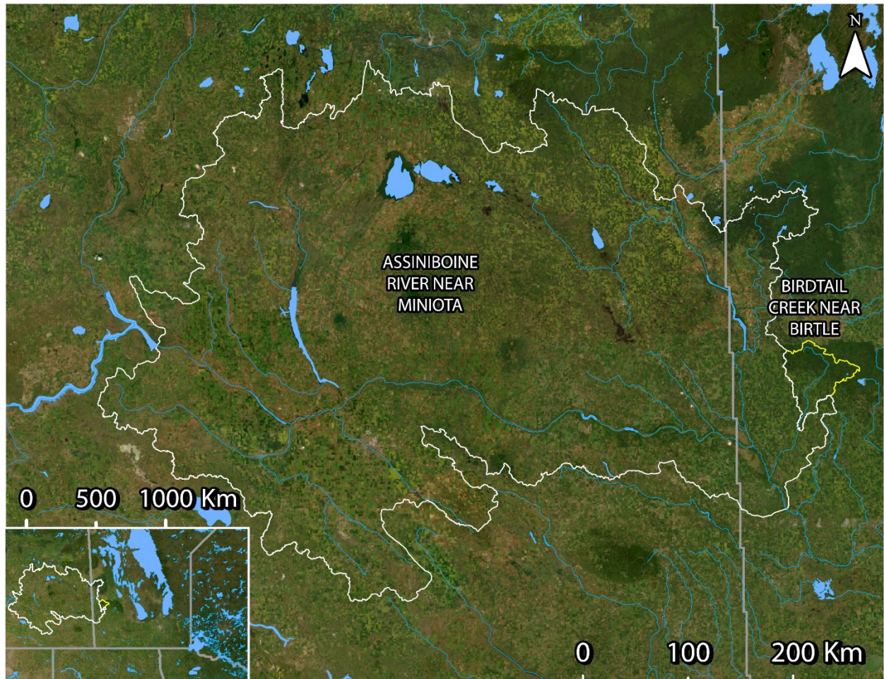
Supplemental Figure 3: Incremental drainage area in white and upstream drainage area in yellow. Incremental values are calculated by subtracting “Birdtail River near Birtle” from gross “Assiniboine River near Miniota” values.
