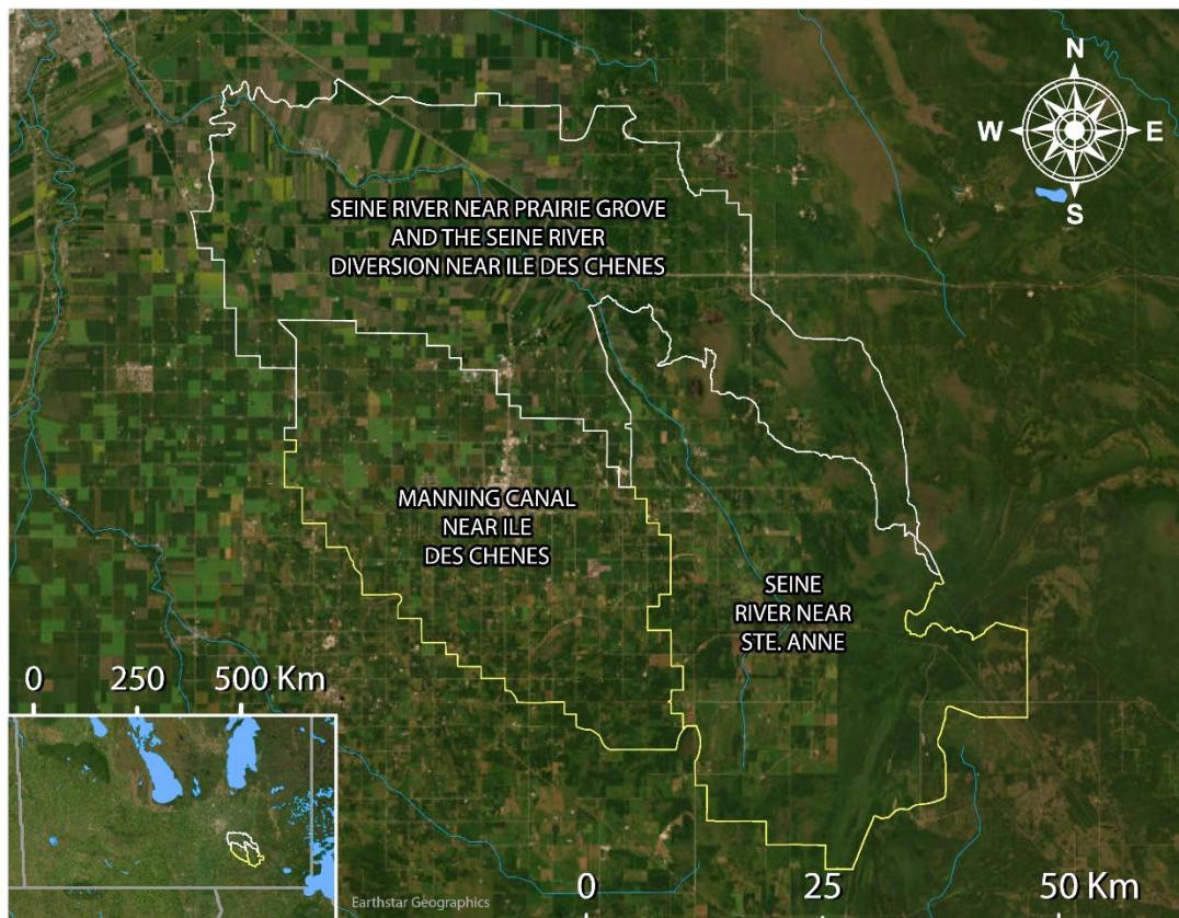
Supplemental Figure 1: Incremental drainage area in white (combined area of WSC stations Seine River near Prairie Grove and the Seine River Diversion near Île-des-Chênes) and upstream drainage areas in yellow (Manning Canal near Île-des-Chênes and Seine River near Ste. Anne). The combined incremental drainage area for Seine River near Prairie Grove (05OH009) and Seine River near Île-des-Chênes (05OE011) was calculated by adding the former two gross drainage areas together and subtracting the upstream gross drainage areas of Manning Canal near Île-des-Chênes (05OE006) and Seine River near Ste. Anne (05OH007).
