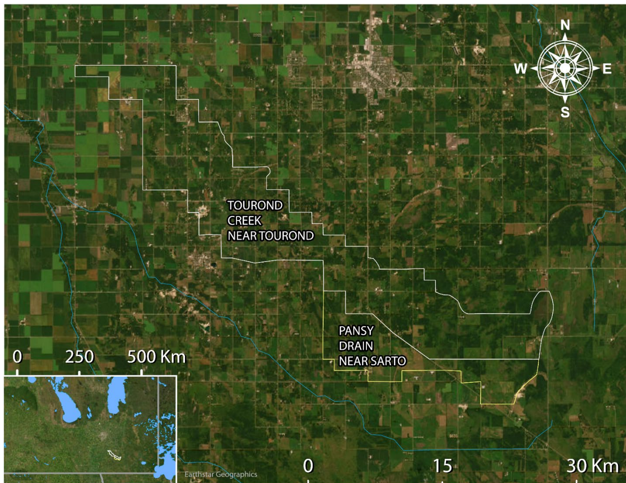
Supplemental Figure 2: Incremental drainage area in white and upstream drainage area in yellow. Incremental loads are calculated by subtracting gross “Pansy Drain near Sarto” values from gross “Tourond Creek near Tourond” values.
